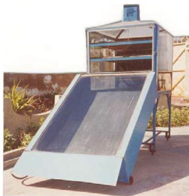
Figure - 6: Solar Dehydrator
