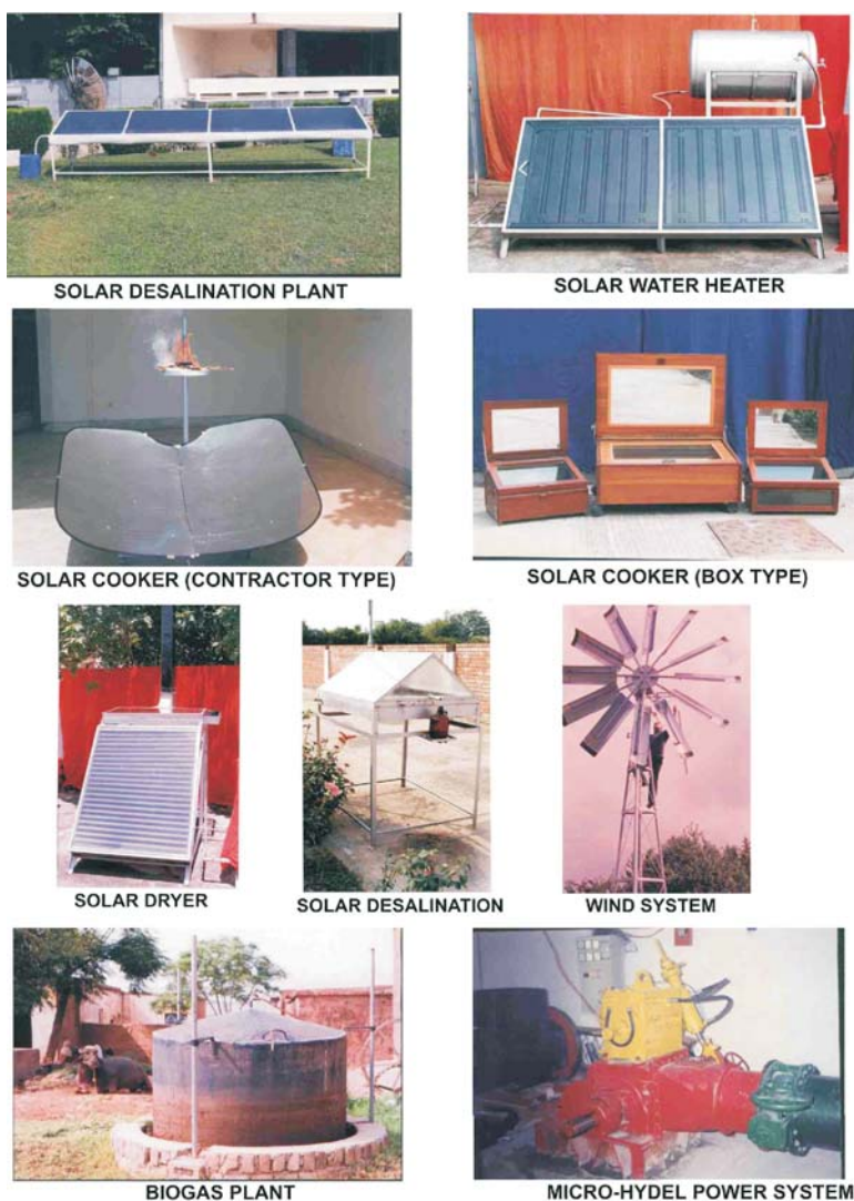
Figure - 2: Solar Thermal, Wind, Biogas and Micro-hydel Appliances from PCRET
